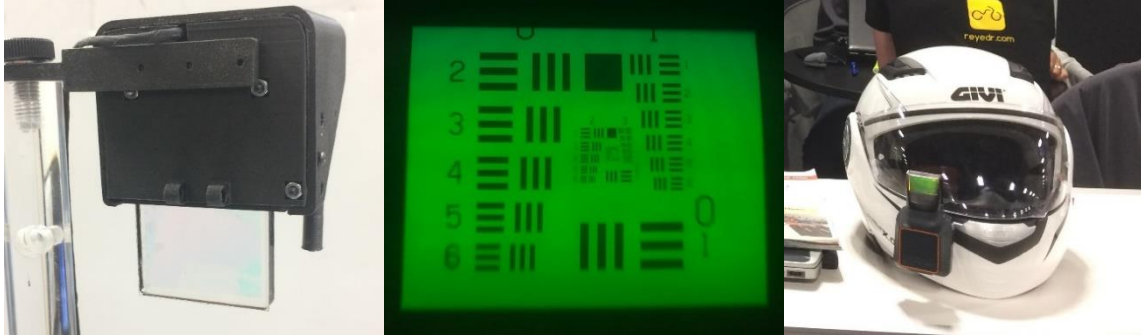
Figure 2. From left to right: Luminet monochrome HMD demo, virtual image by demo, and RGB HMD for a motorcycle helmet.
